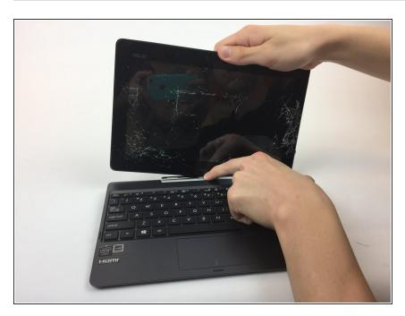
Detach the keyboard from the screen by depressing the silver button the hinge and pulling upwards on the tablet.
