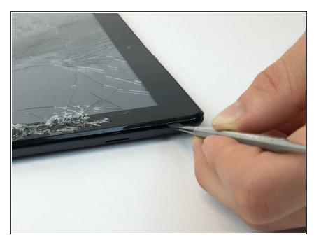
Take the tablet-portion of the device and carefully pry the screen open using either the plastic or metal spudger. Each interior clip needs to be released from the edges.
