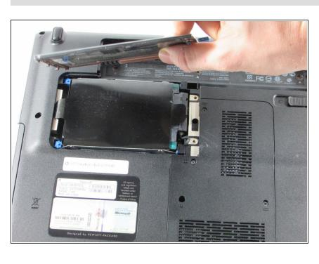
After removing the two screws securing the Hard Drive to the bottom case, remove the panel to reveal the hard drive.
