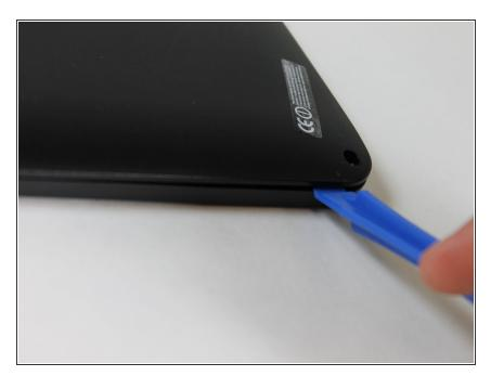
Using the plastic opening tool, remove the back cover of the device.
