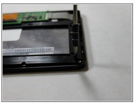
Remove the eleven screws that hold the screen to the base. Eight are .15 mm and three are .11 mm.
