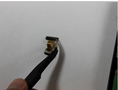
Use a pair of small tweezers to gently pull the camera connector out of the motherboard.
