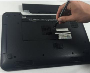
Remove the 5 mm Phillips # 0 screw in the middle of the device.
