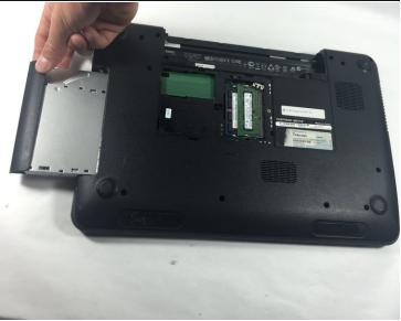
Insert a small screwdriver into the hole and slide the optical drive away from the center of the device. This will slide the optical assembly out from the side of the device.
