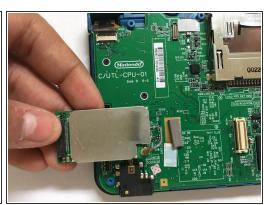
Lift the Wi-fi Board off of its socket.(you can also put this back.)
