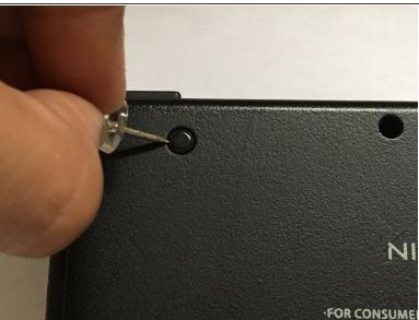
Remove the rubber blocking the screws on the Dsi XI with a push pin don't hesitate about it.
