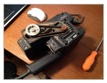
Remove the screw on the very top of the device (side with SKIL logo)
