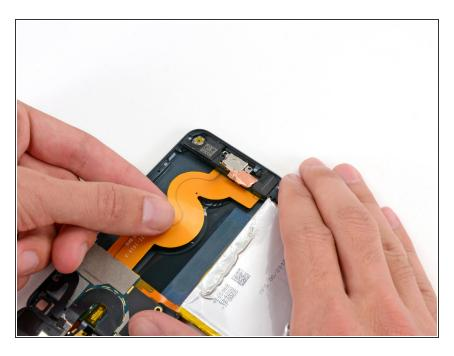
Gripping the large ribbon cable, gently pull the Lightning connector assembly out of the bottom of the case.
