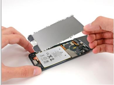
Lift up the LCD plate to remove it
