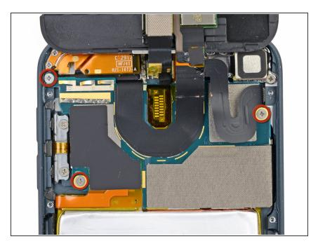
Remove three 1.6 mm #00 Phillips screws that are securing the logic board onto the rear case.
