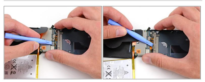
Use a plastic opening tool to disconnect the display cable from its socket.
