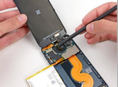
Get a spudger and use the flat end of it to take out facing camera out of its socket in the display assembly.
