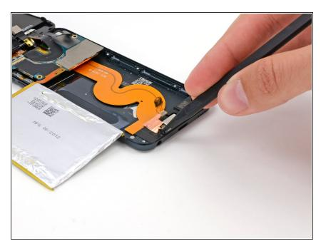
Use the tip of a spudger to peel back a piece of tape covering a screw on the side of the headphone jack.
