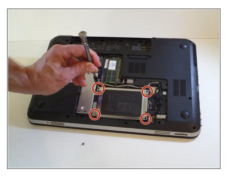
Use the PH 1 screwdriver to remove the four 3.5 mm screws securing the hard drive.
