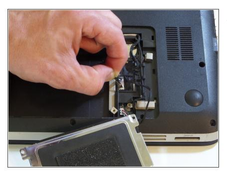
Unplug the hard drive wire to detach the hard drive.
