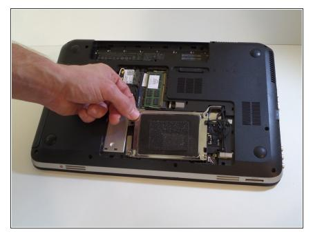
Lift the corner bracket to remove the hard drive.
