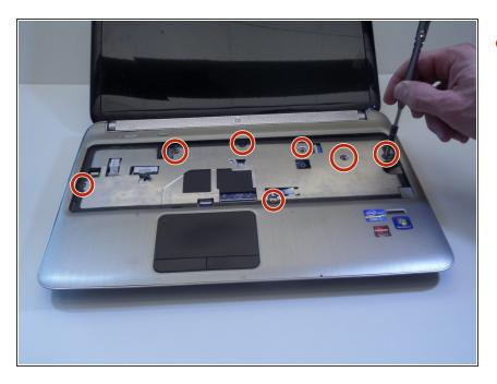
Remove seven 4mm pannel screws with PH 1 screwdriver.
