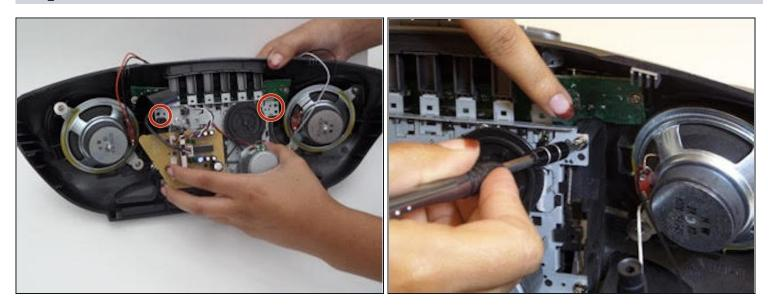
• Facing the inside of the front panel, on the corners of the grey plate, there are four screws. Unscrew these with a phillips 1.
