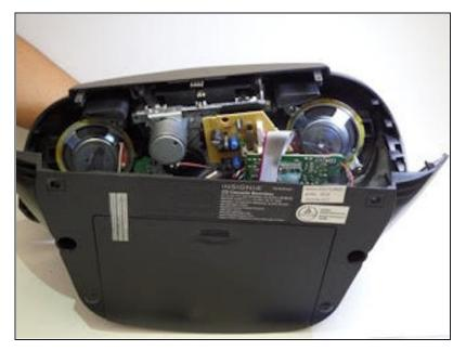
Face the bottom of the opened boombox, and detach the front panel from the back in the following order:
