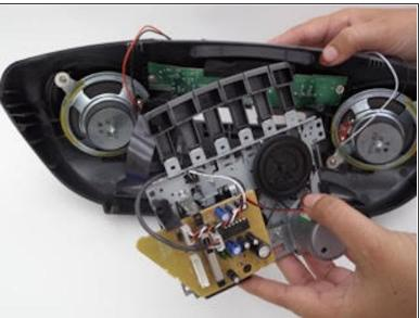
Face the inside of the front panel. Push the buttons down gently to slide the cassette player unit out.
