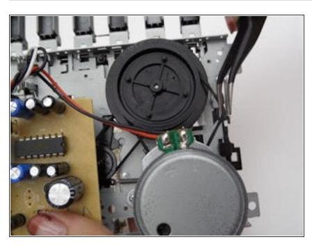
On the back of the unit to the right of the motherboard and between the motor and black circle, there is a rubber band that allows the spinning wheels to spin the knobs. Using tweezers, remove the rubber band and replace it. To reassemble your device, follow these instructions in reverse order.
