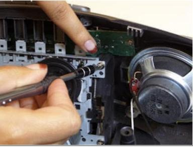
Facing the inside of the front panel, on the corners of the grey plate, there are four screws.
