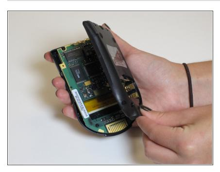
Close again like a book, and lay it gently into the front panel. Make sure the screen is facing outwards of the front panel.
