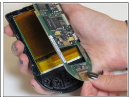
Remove rear cover by gently lifting it up from the bottom. To remove the front cover, flip the device over, and then separate the screen/circuit board from the cover.
