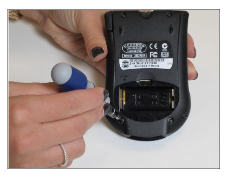
Using a Torx 5 screwdriver, remove the four screws located on the rear cover of the device by turning counterclockwise. Set aside screws.
