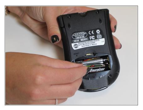
Remove the batteries.
