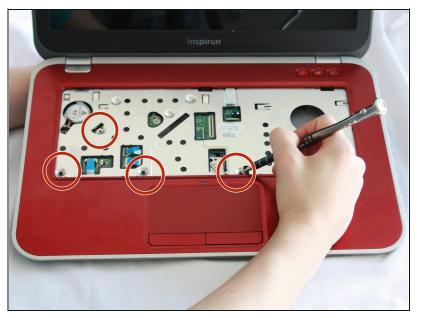
Use J0 Bit screwdriver to remove all four 6 mm Phillips screws.
