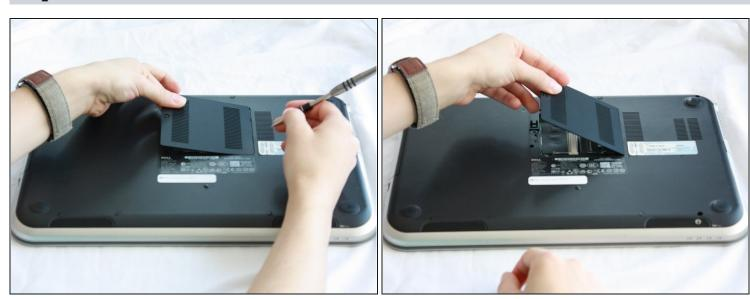
• Lightly lift the RAM cover up and at an angle, away from the computer.
