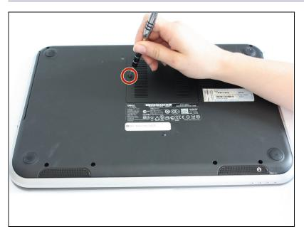
Use a J0 bit tipped screwdriver to unscrew the one 6 mm Phillips screw on the RAM cover.
