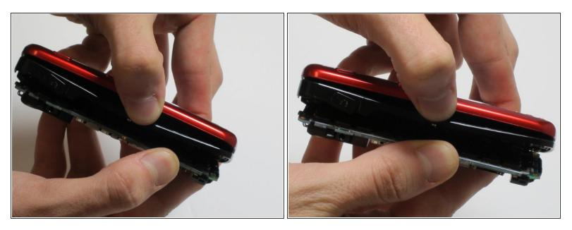
• Remove the casing from the back of the device.
