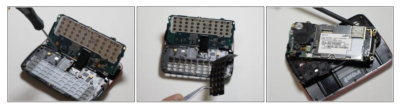
• Last, unscrew the remaining screws and remove the keyboard padding, exposing the motherboard.
