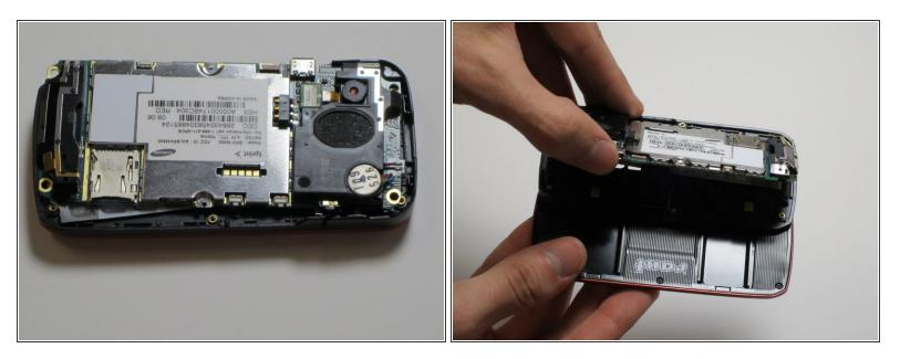
Next, separate the back component from the keyboard and screen, exposing the middle of the phone and keyboard pad.
