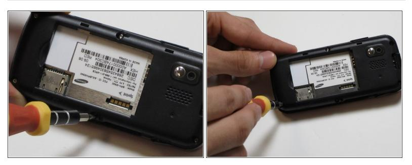
• Using a Phillip's #00 screwdriver, unscrew the 6 screws located on the back of the device.
