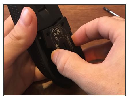
Insert your thumb and index in the two mouse holes and gently pry the sensor assembly out from its socket.
