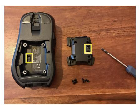
The sensor assembly is linked to the mouse body with a 10-pin Steelseries custom connector.
