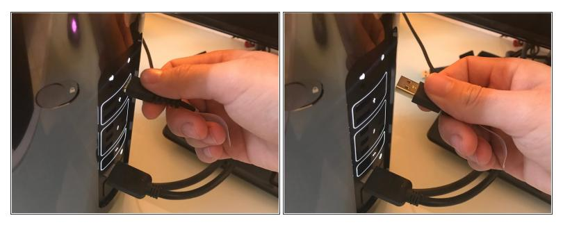
• To avoid electronically damaging either your computer or your mouse, unplug the usb cable from its socket.
