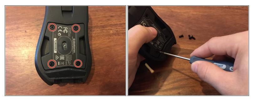
Use a Philips #0 screwdriver to remove the four screws that are keeping the mouse sensor assembly sealed.
