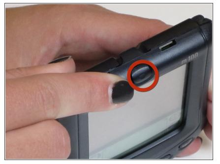
Once positive that the batteries are installed correctly, press the on/off located at the top center of the device.
