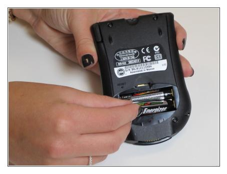
• Check the type of batteries to be sure they are both AAA batteries.
