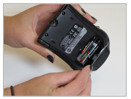
Take the battery cover off by pushing down on the tab and lifting off.
