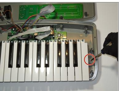
Remove the two highlighted 10 mm M3 galvanized machine screws using the J1 head fro the iFixit Tool Kit or a comparable tool.
