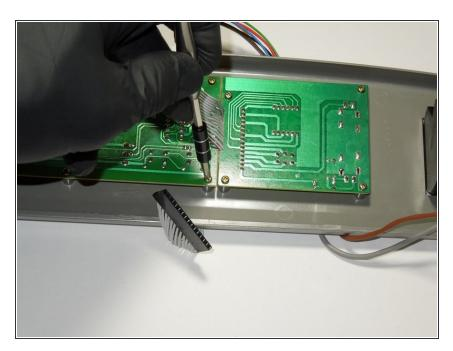
Remove all five screw in any order with the J1 screwdriver head from the Ifixit tool kit.
