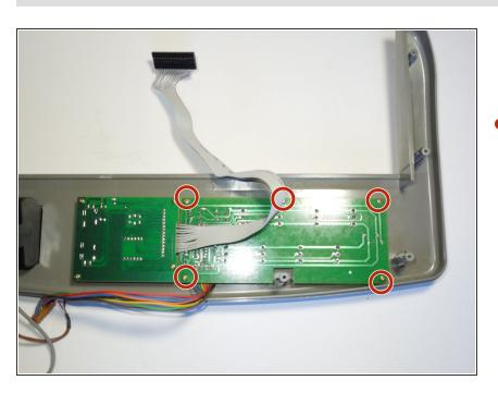
This is the location of the tuning potentiometer circuit retaining screws, 5 each 10mm long M3 galvanized Philips head machine screws
