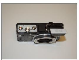
Use a plastic opening tool to lift off the top panel.
