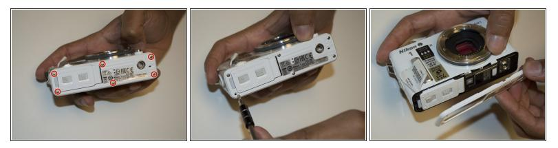
Using the Phillips PH00 screwdriver, remove the six 4.0mm screws marked in red. Then remove the panel cover by lightly pulling it off.
