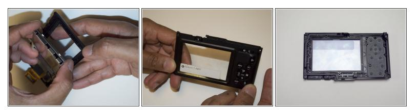
• Remove the back panel apart from LCD screen.
