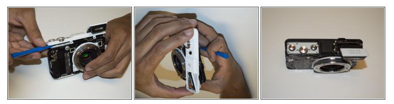
• Use a plastic opening tool to lift off the top panel.
