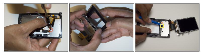
Lift the rainbow cable to have access to the 3.1mm screw beneath it and unscrew it with a Phillips PH00 screwdriver.
