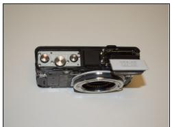
• Use a plastic opening tool to lift off the top panel.
