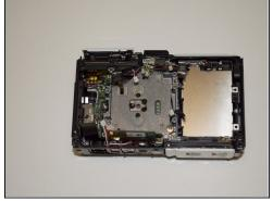
Carefully remove the motherboard from the main camera body and replace it for a new one.
