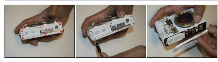
Using the Phillips PH00 screwdriver, remove the six 4.0mm screws marked in red. Then remove the panel cover by lightly pulling it off.
