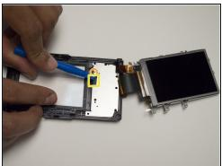
• Lift the rainbow cable to have access to the 3.1mm screw beneath it and unscrew it with a Phillips PH00 screwdriver.
