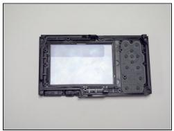
• Remove the back panel apart from LCD screen.
