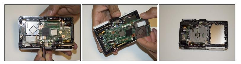
• Carefully remove the motherboard from the main camera body and replace it for a new one.
