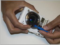
Squeeze the O-ring under the lens support to push out the O-ring. Use a plastic opening tool to get under the O-ring, and slowly work around the metal lens support to pull the O-ring completely out.
