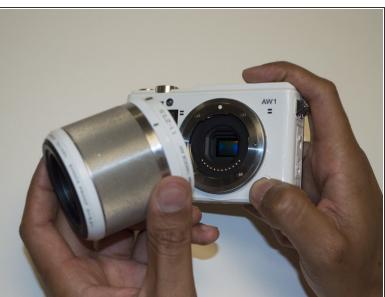
Press and hold the lens release button, twist the lens in a clockwise motion, then pull it off of the camera.
