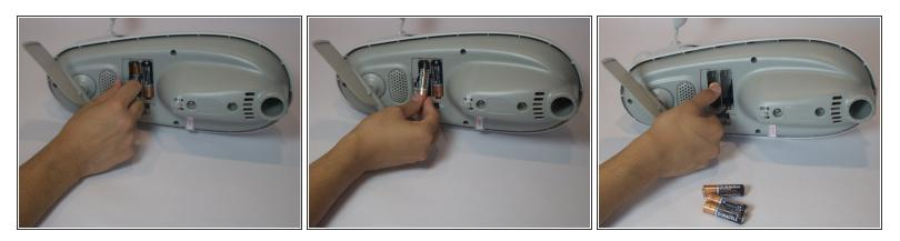
• Once the batteries are removed, it is safe to proceed.
