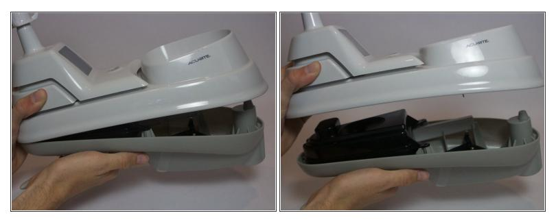
Gently lift the top section of the weather center away from the base. With all the screws removed it should lift off easily.
