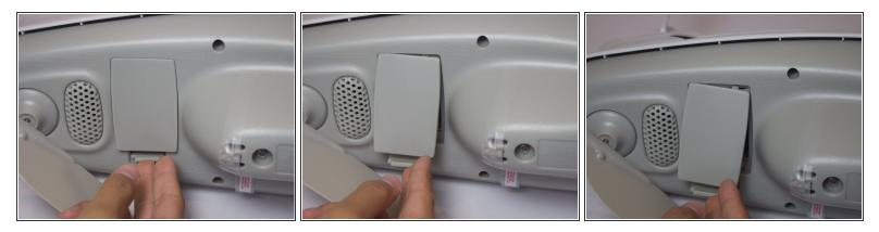
• Remove the battery compartment lid by lifting upward.
