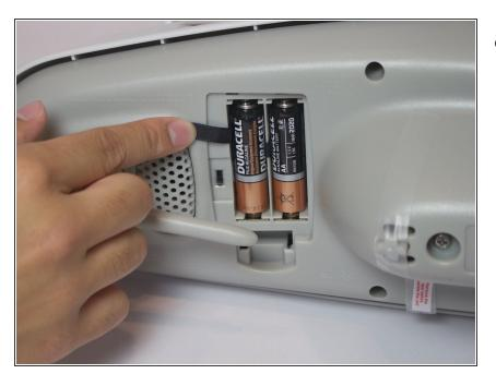
Pull the ribbon to eject the 2 X AA alkaline batteries.
