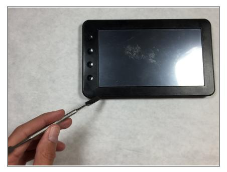
Wedge the metal spudger in between the faceplate and the body of the tablet.
