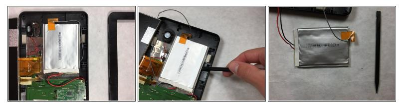
• Carefully pry the battery away from the body of the tablet using the plastic spudger.
