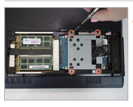
Use the J1 screwdriver to unscrew the four 3mm Phillips screws on the hard drive.
