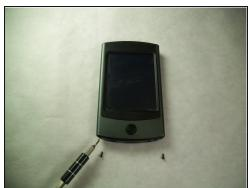
• Using the screwdriver with the J00 bit, remove the two 4.8 mm Phillips screws.
