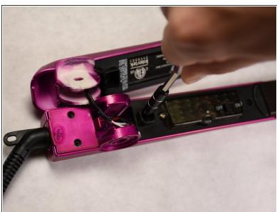
Using a Philips head #1 screwdriver remove the two 6mm black screws on both sides of the dial panel cover.
