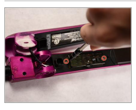
Using a Philips head #1 screwdriver remove the two 4mm silver screws on both sides of the dial panel cover.
