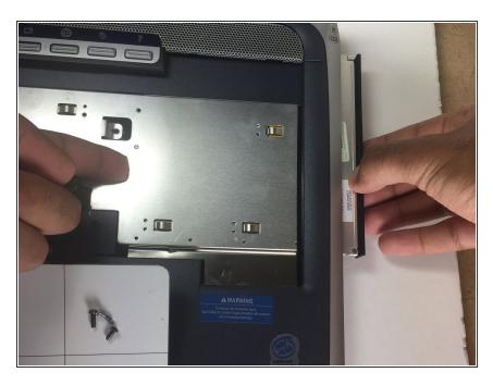
After the screws have been removed, use one finger to push the CD Rom out while the other hand is simultaneously pulling the CD Rom out.
