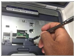
• Unscrew three screws from under the keyboard. The keyboard must be removed for this process.
