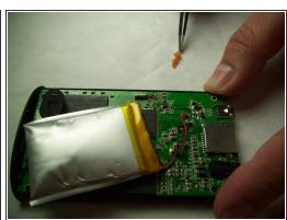
Using the straight tweezers, remove the plastic coating on the wires.
