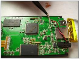
• Using the soldering guide, desolder the battery connections.
