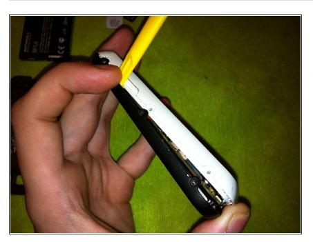
Use the pry tool and insert in between the black and white plastic.
