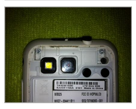
• Remove the two torx screws in each corner.
