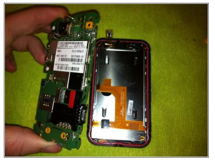
• Lift the logic board out of the phone revealing the LCD.
