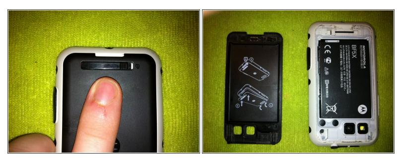
• On the back there is a slider that locks the back cover on slide this over to unlock it.
