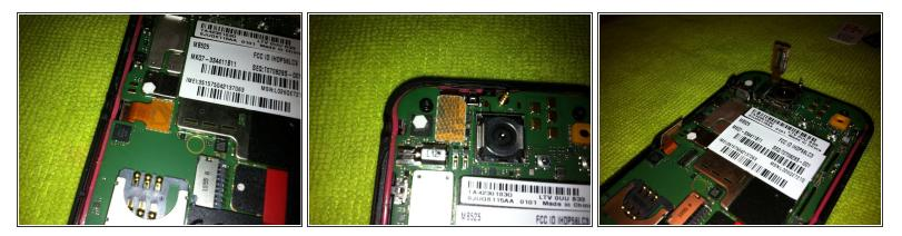
• Use the pry tool and detach the digitizer cable and LCD cable from the board.
