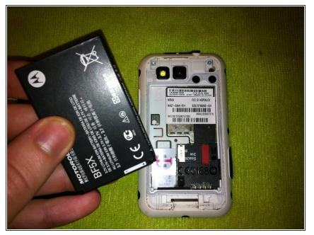
• Remove the battery and sim card as well as the micro sd if one.
