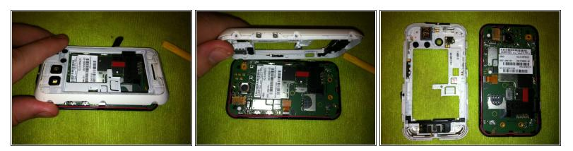
Remove the the back case (white section) revealing the logic board.
