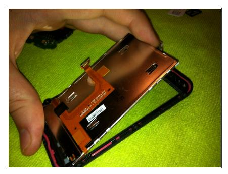
• Use pry tool to gently lift the LCD out of the phone revealing the digitizer.
