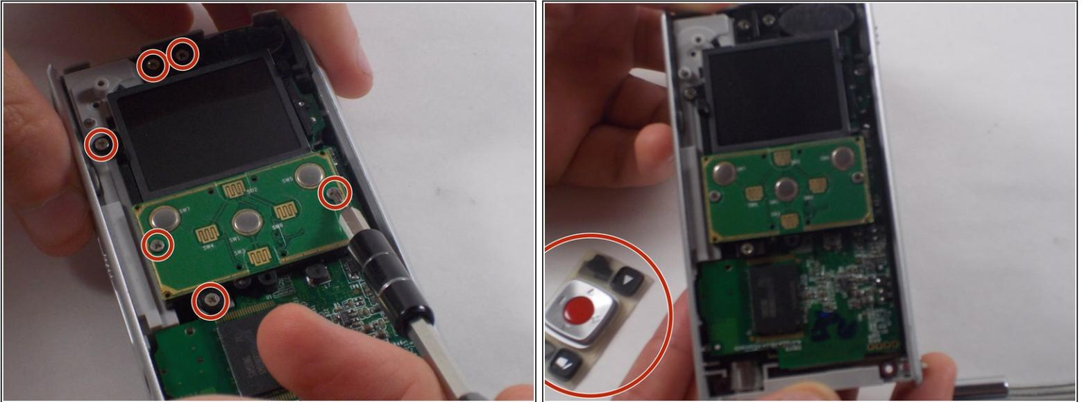
**i** When removing the back panel, the rubber buttons will become loose and likely fall off the board. This is normal and can easily be placed back on the board once finished.
