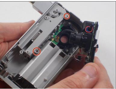
Unscrew the single 1mm screw from USB housing unit.
