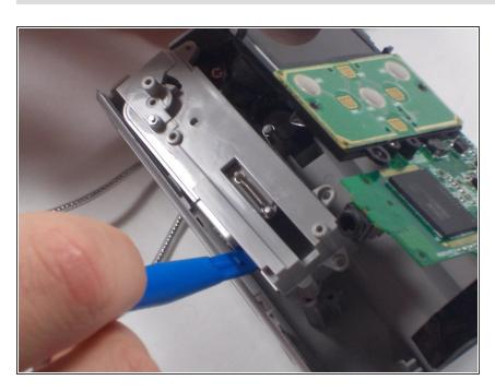
Gently pry out the USB housing unit with the Ifxit Opening Tool.
