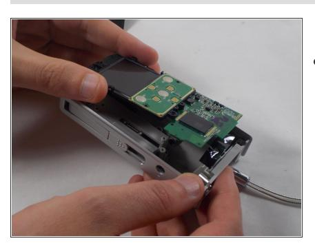
Gently separate the circuit board from the casing.
