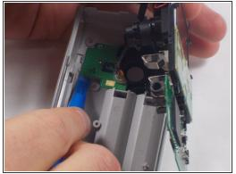
Remove the two 1mm screws and separate the circuit board and camera from the plastic casing.
