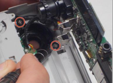
Unscrew the 2 1mm screws and gently separate camera wires from plastic casing.
