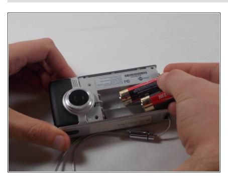
Remove the batteries
