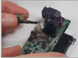
With tweezers, remove the microphone and USB connections.
