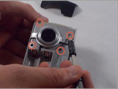
Remove the six 1mm screws from the back and upper casing with the Phillips Head screwdriver.
