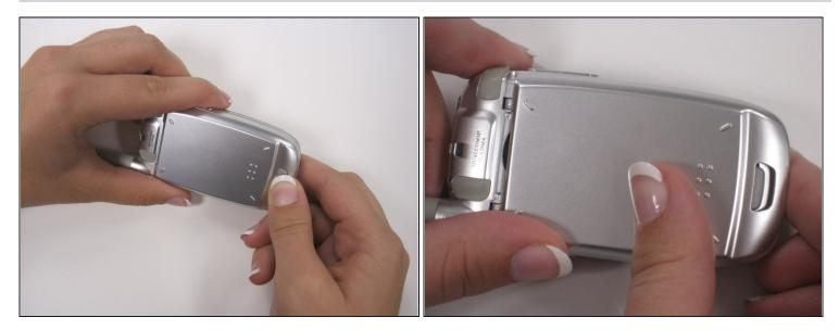
• Remove the back panel by first pressing and holding the gray button on the back. While doing that also press and slide the panel down and off.
