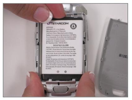
• Carefully remove the battery from the phone by prying the battery from the top.
