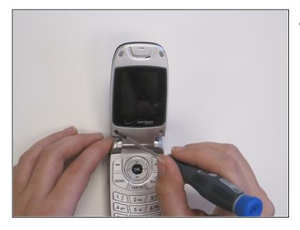
• Remove the four screws from around the phone's screen with a Phillips screwdriver.
