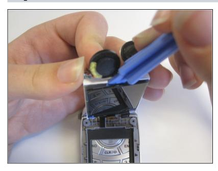
• Pry the circuit board off of the screen with the opening tool.
