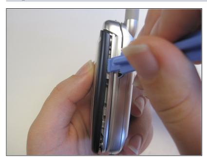
• Pry the top cover off the phone with a plastic opening tool.
