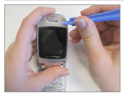
• Remove the rubber plugs from the screw holes around the screen with the opening tool.
