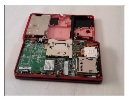
After you have unscrewed all of the screws. Carefully remove the back with a spudger.
