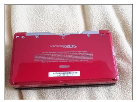
Take out the 4 screws on the back of the system using a Phillips #00 Screwdriver.
