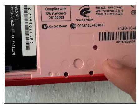
You will see small black screws in nine different holes. make sure you use the right screwdriver and remove them. Also remove the one silver screw that holds the game cartridge slot.
