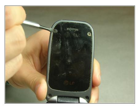
Remove the four rubber covers from the front screen using a metal spudger.
