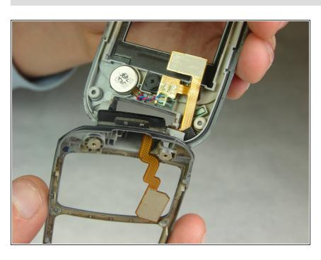
You can now carefully pull apart the phone casing at the hinge by separating them at the left side of the hinge. To reassemble your device, follow these instructions in reverse order.
