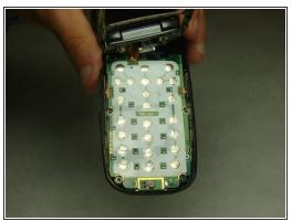
You should notice that the number pad is loose and can simply be taken out of the open phone casing.
