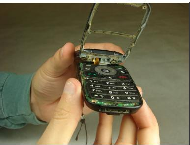
Once you have worked your way around the perimeter of the phone, you will have access to the components in the bottom half assembly.
