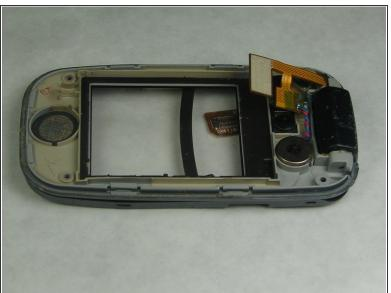
Grip the screen and ear speaker connected to the screen via red and black wires, and carefully pull the screen away from the screen assembly.
