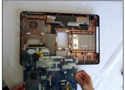
• Lift the circuit board out of the back panel and turn it over so the fan is facing up.
