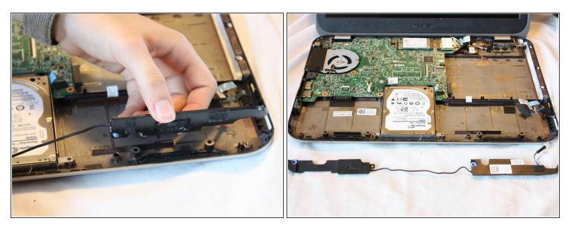
• Using a rolling motion, remove the speakers from the base of the computer
