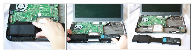
• Lift the tiny black tab and pull the battery out at a slight angle.
