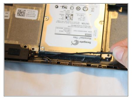
Release the wire connecting the speakers from the securing clips by pulling them upward.
