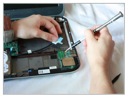
• Use a J0 Bit screwdriver to remove the two 6 mm Phillips head screw located on the daughter board.
