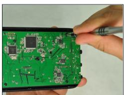
Remove the four screws that hold the motherboard in place.
