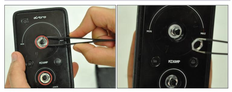
Using tweezers, remove the spacer nuts and washers from each dial post.
