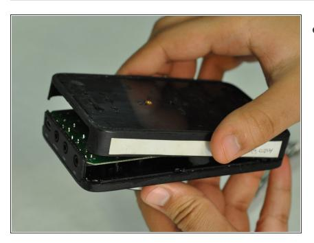
Gently lift the rear casing from the device.
