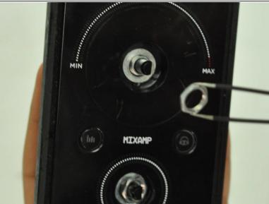
• Using tweezers, remove the spacer nuts and washers from each dial post.
