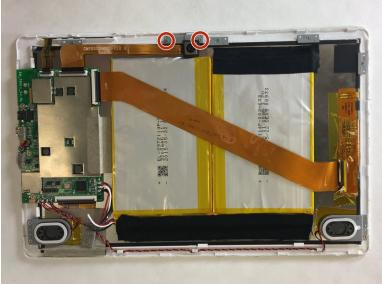
Use a #00 Phillips head screw driver to remove the two screws that hold the camera down to the front case.
