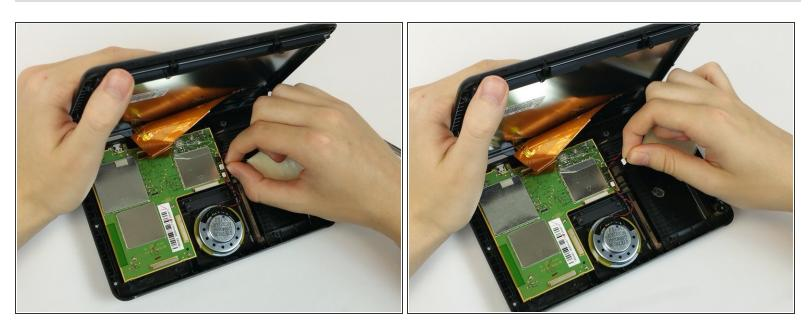
Grasp the battery wire near the motherboard and lift upward to detach the connector.
