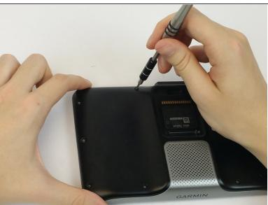
Using a Torx T6 Screwdriver, remove the ten 7mm screws from the back panel.
