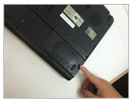
• Locate the RAM storage space on the back of your Toshiba Satellite.
