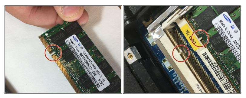
Be sure to match each RAM components female insert, with the laptops male insert during reassembly. If you do not reinstall the components correctly your motherboard may fry.
