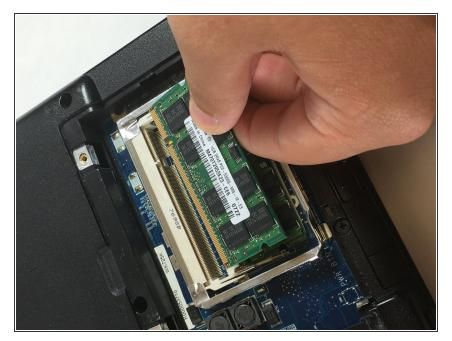
Gently pull and remove the RAM component, and repeat for the second component laying underneath the first.
