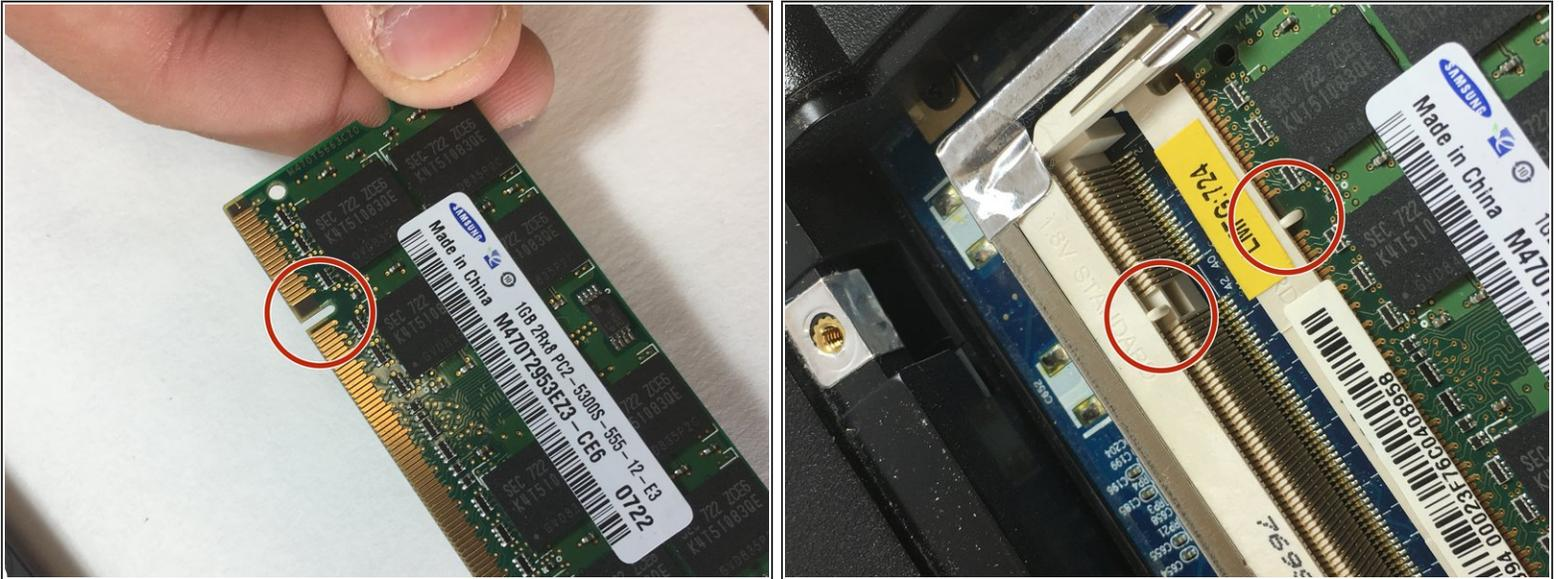
**!** Be sure to match each RAM components female insert, with the laptops male insert during reassembly. If you do not reinstall the components correctly your motherboard may fry.
