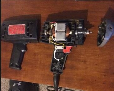
• Once you have unscrewed all of the screws you now pull the metal head off. After you have pulled the metal head off then you pull the other half of the drill case off.
