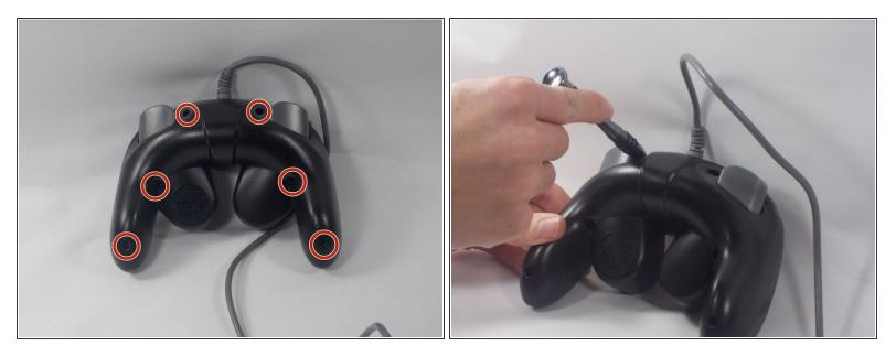
Loosen and remove the 6 screws located on the back of the controller using your Phillips Screwdriver.
