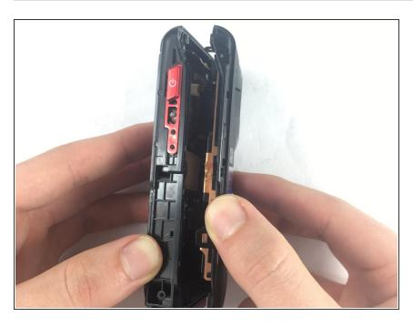
Separate the front and back casing.
