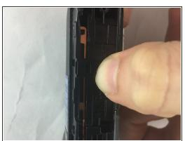
Lift the two plastic tabs on the left side of the LCD screen and the single one on the right side on the black casing to open the device.
