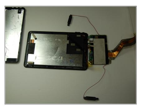
Once faulty speakers have been unscrewed, disconnect the speaker and attach the new speaker to the mother board.
