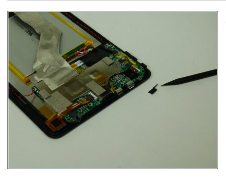
Once the faulty power button is removed, follow the directions in reverse order to reassemble the device.
