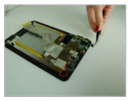
Using tweezers, gently grab the power button and pull it out from the tablet.
