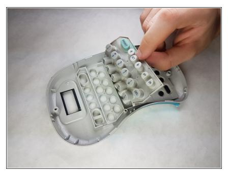
• Peel the keypad contacts up from the plastic casing.
