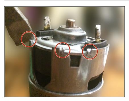
When re-assembling, I had to clamp together the bearing housing and motor in a vice while I tapped the 8
